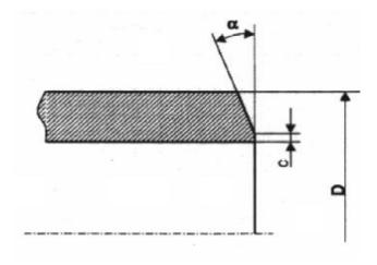
Figure 1 — Tube end bevel
